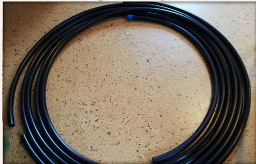
1. Pe-Rohr 25mm
